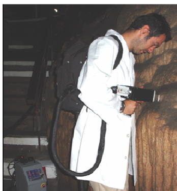
Figure 2. Photo of the man-portable laser system during the field campaign carried out in the Nerja Cave.
