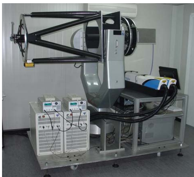
Figure 1. Photograph of the LIBS sensor for stand-off analysis of materials.
