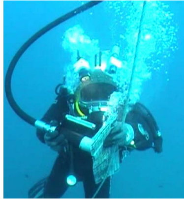
Figure 2. Photo of the LIBS probe taken during a LIBS analysis underwater (30 m).
