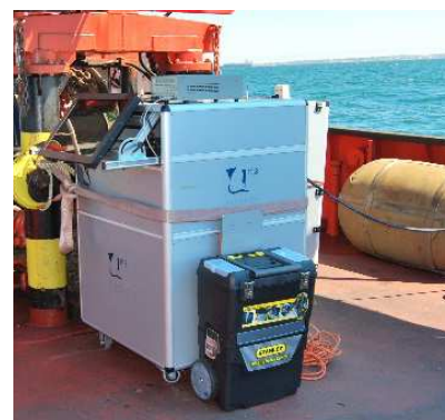
Figure 1. Schematic diagram of a portable LIBS instrument used for underwater cultural heritage analysis.
