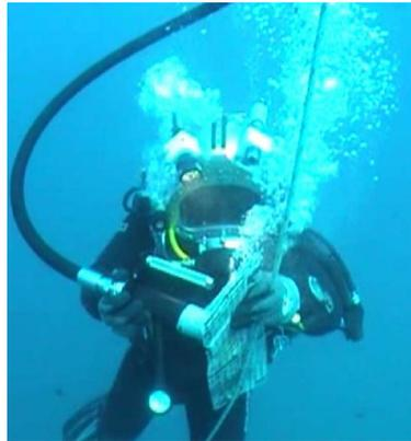
Figure 2. Photo of the LIBS probe taken during a LIBS analysis underwater (30 m).
