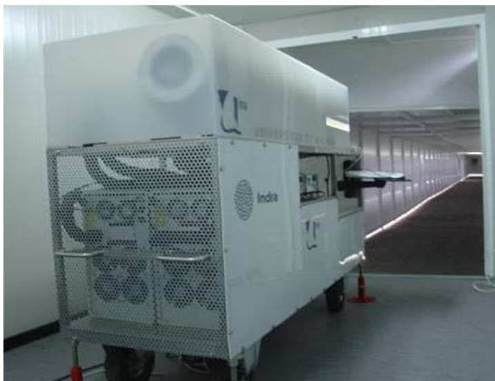
Figure 3. Photograph of the Raman sensor (also configurable for LIBS) used for the analysis of materials at a distance and view of the experimental corridor (50 meters total length).
